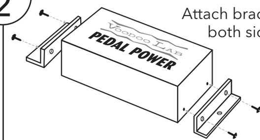
**Step 3** Align Pedal Power brackets to mounting holes.
